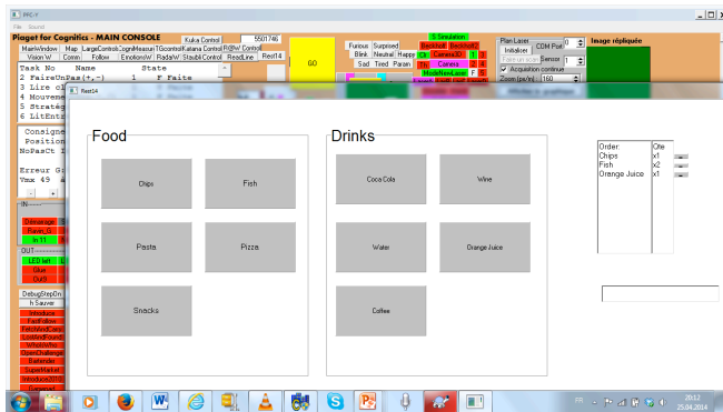
Fig. 5. Example of robot RH-Y form for interactively taking orders in a restaurant. Orders may be taken with a tactile screen or given vocally.
